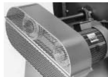
BELT GUARD—STANDARD ARR. 9 Bearing side is enclosed. Not available unless Cincinnati Fan mounts motor.
